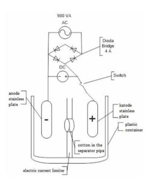
Figure1. Seawater Electrolysis Instrument
