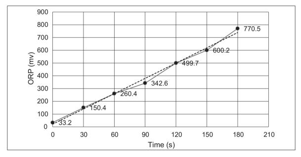
Figure 2. Relationship between ORP and time during electrolysis
