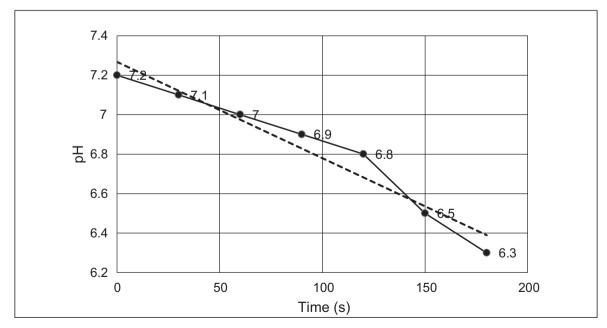
Figure 3. Relationship between pH and time during electrolysis
