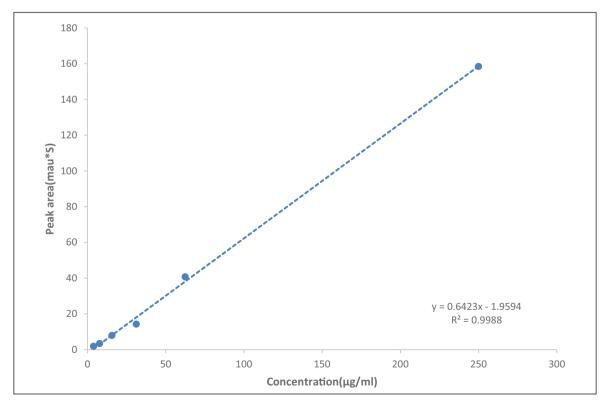
Figure 1: The calibration curve of standard vitamin A
