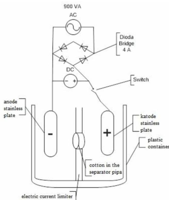
**Figure 1.** Seawater Electrolysis Instrument
