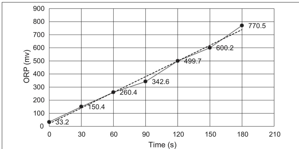
**Figure 2.** Relationship between ORP and time during electrolysis
